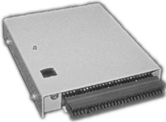
Fig 3.5 The Plus D in its Datel case. The little red button froze the Spectrum so you could save a snapshot of your game to disk.
